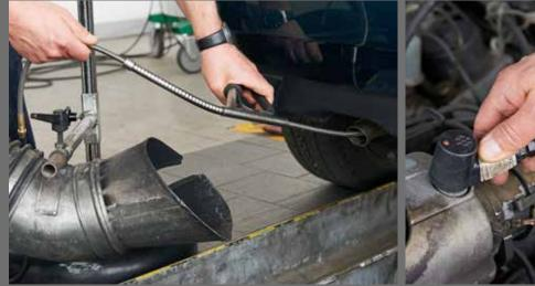
Cars need to undergo an exhaust emissions test every two years in Germany. This involves sensors being attached to the exhaust and the cylinder head.
