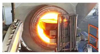
Furnace with oxy-fuel combustion system
