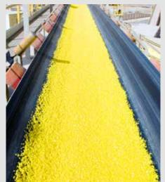
Granulated sulphur is used as a raw material for sulphuric acid.
