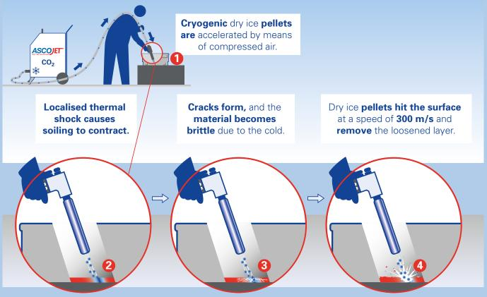
Dry ice blasting technology is used after testing in the engine development department to remove silicon residue, oil, grease, combustion residue and the like from engine components in a gentle cleaning process.
