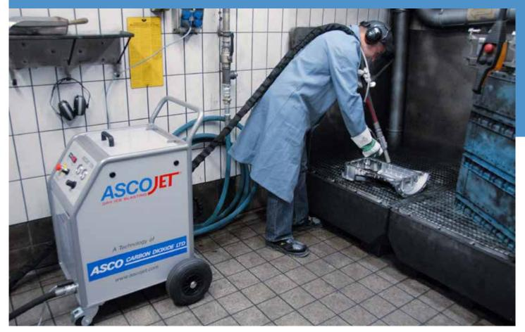
Cleaning an engine component with dry ice blasting technology from ASCO Carbon Dioxide
