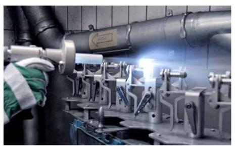
The gun light fitted to the gun illuminates the narrow annular groove during cleaning.
