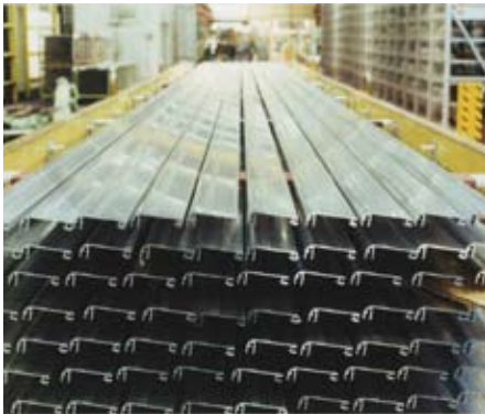
The INCAL process increases productivity during aluminium extrusion.
