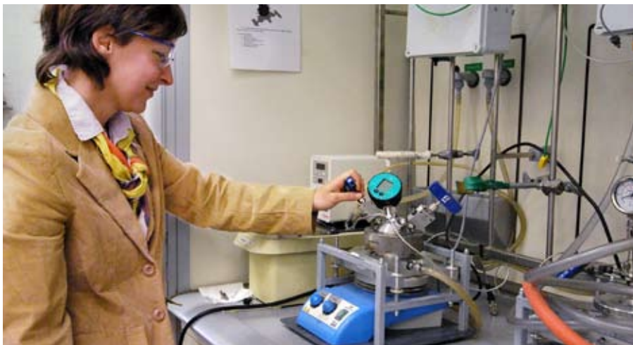
Dr. Edit Székely, a member of the SFE research team, adjusts the settings on the CO 2 reactor in the SFE laboratory.
