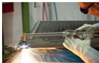
The ESSEN hand cutting torch for flame cutting material of up to 500 mm in thickness and for gouging
